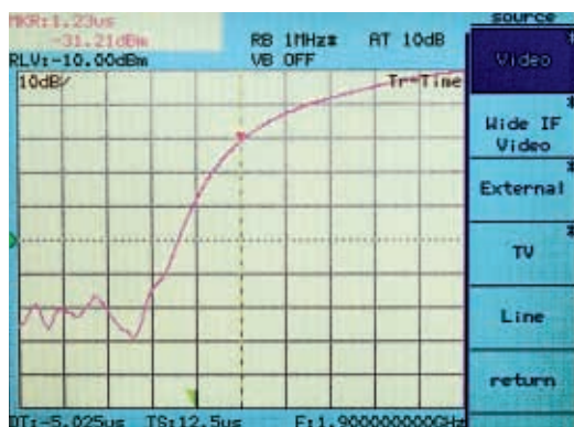
High-speed time-domain measurement (TS=12.5 \mu\text{s} )
