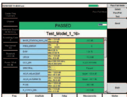
The Modulation Summary screen shows critical transmitter performance parameters in table format.
