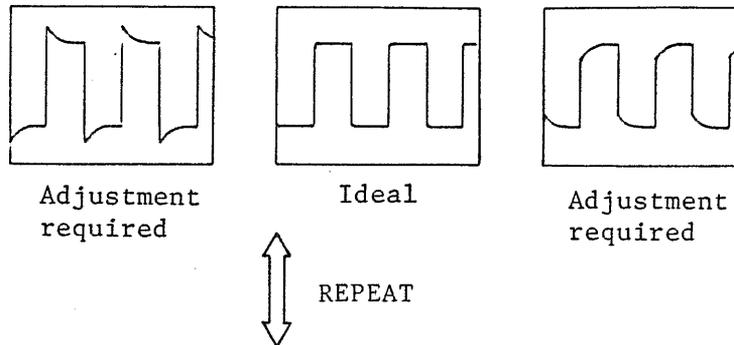
Adjustment of HF COMP (C117, C218) of preamplifier
