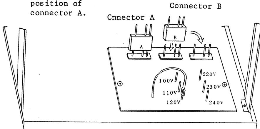
Connect the selector cord to the corresponding pin.
