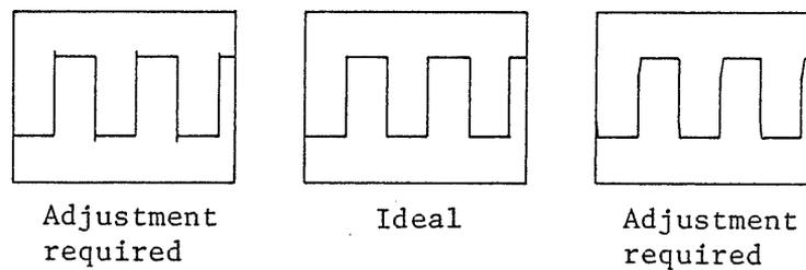
By the above adjustment, the square wave characteristics also adjusted.
